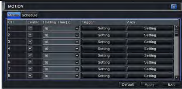
Fig 4-4 Motion detection interface
